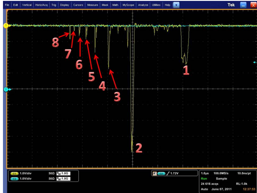
Figure 2.8 Picture of oscilloscope traces showing argon ion peaks \text{Ar}^+ through \text{Ar}^{8+} inside the interaction chamber, 42 mJ pulse energy.
